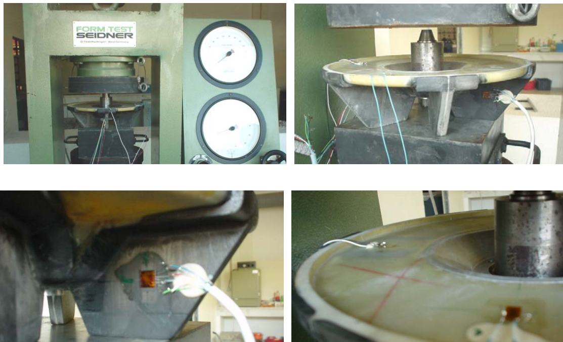
Figure 7. Hydraulic press and gauges implementation.
