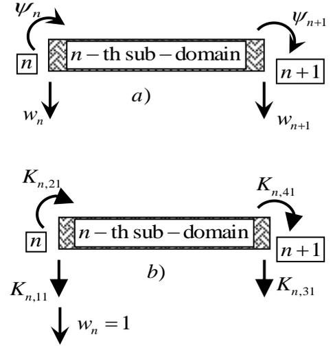
Figure 5. a) Degrees of freedom, b) construction of the local dynamic stiffness matrix of the  $n$ -th sub-domain.
