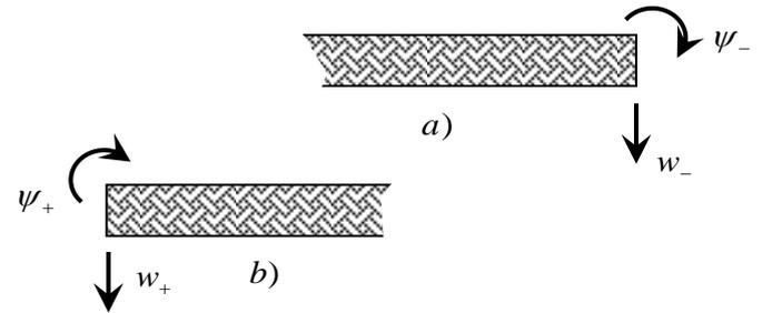
Figure 6. Degrees of freedom of semi-infinite sub-domains: a) negative, b) positive.
