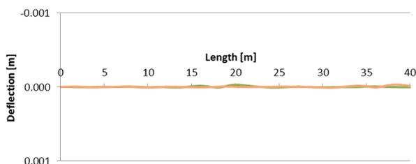
Figure 7. Deflection of the simply supported beam on an elastic foundation, initial 40m of the full length, deflections related to mass position at 18m and 36m.
