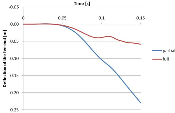
Figure 2. Deflection of the cantilever free end, “partial” means that some terms were omitted as in [8], “full” means that all terms are included.
