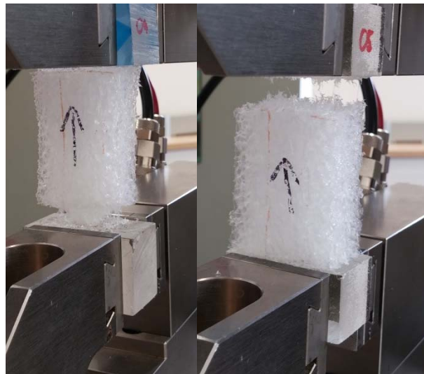
Figure 4. Failure of BM specimens in tension
