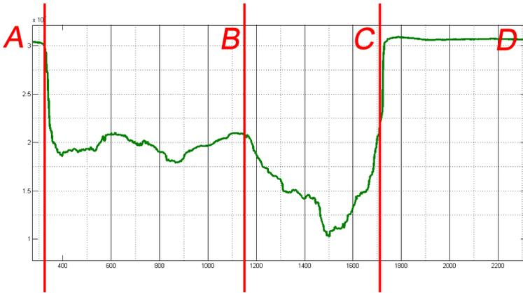
**Fig. 5.** Y axis read by the accelerometer (Median). A: standing, A-B: seating, B-C: seating more vertically, C-D: standing. [Signal length: 1m 20s at 25Hz] (Vertical axis: amplitude; Horizontal axis: sample).
