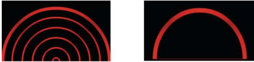
Fig. 3 On the left side is a representation of the GUI for the Manual mode of driving. Each concentric circle represents a different speed (larger is the radius of the semicircle, higher is the velocity). On the right side is the user interface for the Biological condition. A single semicircle enables the user to directly control the direction of the robot and indirectly set the speed of the vehicle
