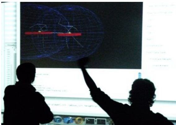
Figure 2: Real-time skeleton extraction from players using OpenNI library.
