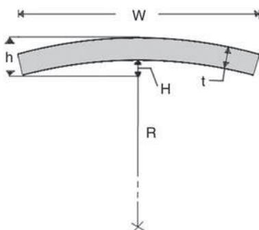
Figure 1. Schematic overview of eggshell curvature measurement method: width ( $W$ ), height across an orthogonal plane of the eggshell ( $h$ ), eggshell thickness ( $t$ ), arc height ( $H$ ) and resulting radius ( $R$ ).
