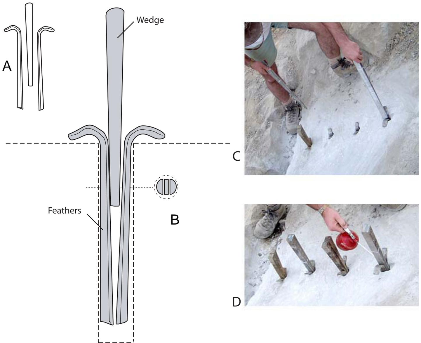
Fig. 3 – Stone-splitters: A- general aspect of the three parts of the stone-splitter; B- cross-section; C- inserting stone-splitters in the rock; D- putting oil between the wedge and the feathers facilitates the sliding.
