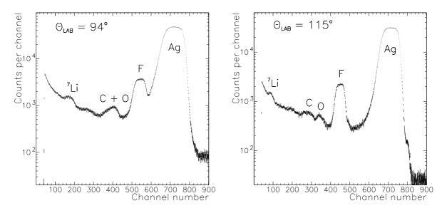
Figure 4.12: The 1.574 MeV  $^4$ He $^+$  backscattering spectra of the LiF-Ag target, measured simultaneously at two different angles,  $\theta_{lab}$ = 94° and 115°.
