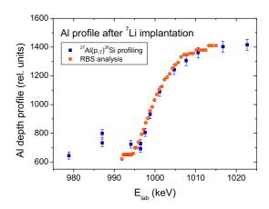
Figure 4.24: Left panel: The excitation function of the  $^{27}$ Al(p, $\gamma$ ) $^{28}$ Si reaction at  $E_{r,lab} = 992$  keV using the Al target before (gray triangles) and after  $^{7}$ Li implantation (blue squares). Right panel: Comparison of Al depth profiles obtained by the  $^{27}$ Al(p, $\gamma$ ) $^{28}$ Si excitation function measurement (blue squares) and RBS measurements (orange circles) – see text for details.
