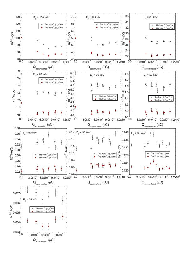
Figure 4.30:  $^{7}\text{Li}(p,\alpha)^{4}\text{He}$  yield  $[N(^{4}\text{He})/Q]$  (red circles) and  $^{6}\text{Li}(p,\alpha)^{3}\text{He}$  yield  $[N(^{3}\text{He})/Q]$  (gray squares) evolution with accumulated charge for the Li metal target. The error bars come from the statistical error on  $N(^{3,4}\text{He})$  counts.
