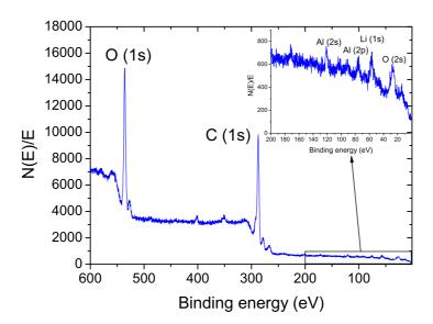
Figure 4.27: Mg  $K_{\alpha}$  X-rays XPS spectrum that shows the detected photo-emitted electrons as a function of the binding energy for the  $^{7}$ Li implanted in Al target surface.
