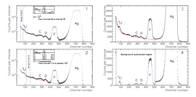
Figure 4.14: The 1.574 MeV  $^4$ He<sup>+</sup> backscattering spectra of the LiF-Ag target, measured at  $\theta_{lab}$ = 115°. Ag plural scattering events (background) subtraction under the  $^7$ Li, C, F and O peaks. The background events are fitted with an  $E^{-\alpha}$  dependence under the  $^7$ Li peak and by two exponentials under the C, O and F peaks. The fitted functions are then subtracted from the spectrum.
