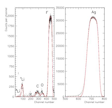
Figure 4.15: The 1.574 MeV  ${}^{4}\text{He}^{+}$  backscattering spectrum of the LiF-Ag target measured at  $\theta_{lab}$ =115° (after background subtraction), and the XRUMP simulated spectrum (red curve).
