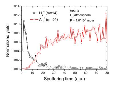
Figure 4.25: The normalized sputtered  ${}^{7}\text{Li}_{2}^{+}$  and  $Al_{2}^{+}$  yield as a function of sputtering time (in arbitrary units) for the  ${}^{7}\text{Li}$  implanted target obtained with a 4 keV  $Ar^{+}$  primary beam in an  $O_{2}$  atmosphere (P =  $1.0 \times 10^{-6}$  mbar). The lines through the data points are to guide the eye only.
