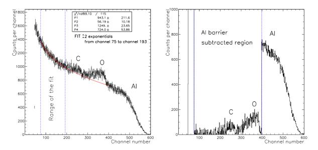
Figure 4.21: The 2.0 MeV  $^4$ He $^+$  backscattering spectra of the  $^7$ Li implanted target, measured at  $\theta_{lab}$ = 140°. The left panel shows the  $\chi^2$  fit to the Al barrier with two exponentials (red curve). The right panel shows the RBS spectrum after subtracting the Al barrier with the fitted exponentials.
