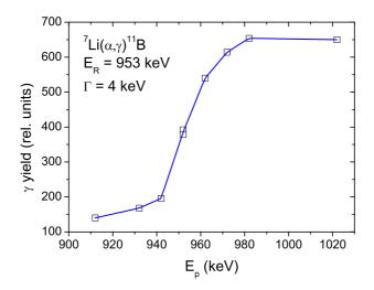
Figure 4.28: The excitation function of the  $^7\text{Li}(\alpha,\gamma)^{11}\text{B}$  reaction at  $E_{r,\text{lab}} = 953$  keV using a  $\text{Pd}_{94.1\%}\text{Li}_{5.9\%}$  target. The line through the data points is to guide the eye only.
