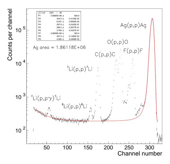
Figure 6.1: The 1021.8 keV H<sup>+</sup> backscattering spectrum of the LiF-Ag target measured at  $\theta_{lab} = 162^{\circ}$ . The red curve shows a  $\chi^2$  fit to the Ag peak with a gaussian plus a gaussian with a low energy lorentzian tail, and a two exponential fit to the continuum produced by the plural scattering events of protons on silver atoms.
