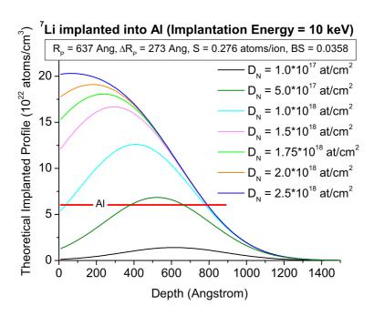
Figure 4.19: Implantated profile evolution with increasing fluence as predicted by eq. 4.10, for <sup>7</sup>Li implantation into aluminium at 10 keV. The red horizontal line indicates the atomic density of pure Al.
