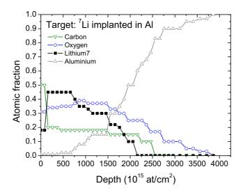
Figure 4.23: Depth profile of <sup>7</sup>Li, Al, O and C predicted by the XRUMP fit to the RBS spectrum of the <sup>7</sup>Li implanted in Al target. The lines through the data points are to guide the eye only.
