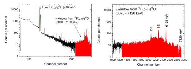
Figure 4.16: Left panel:  $\gamma$ -ray spectrum taken from the LiF-Cu target at  $E_{lab} = 1134$  keV. Right panel: Same spectrum zoomed over the  $\gamma$  window from the  $^{19}$ F(p, $\alpha\gamma$ ) $^{16}$ O reaction. The SE and DE peaks correspond, respectively, to the single escape and double escape peaks of the 6125 keV photo peak.
