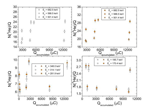
Figure 4.29:  $^7\text{Li}(p,\alpha)^4\text{He}$  yield [N( $^4\text{He}$ )/Q] evolution with accumulated charge for the LiF-Cu target, at different energies. The white and orange data points correspond to the Si detectors at  $124^\circ$  and  $145^\circ$ , respectively. The error bars come from the statistical error on N( $^4\text{He}$ ) counts.
