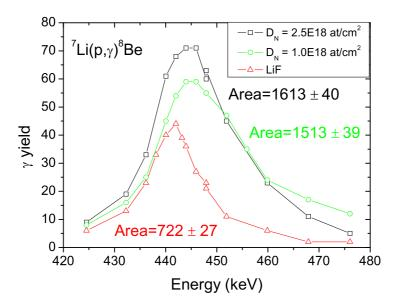
Figure 4.20: The excitation function of the  ${}^{7}\text{Li}(p,\gamma){}^{8}\text{Be}$  reaction at  $E_{r,\text{lab}} = 441.4$  keV using the two implanted targets and a vacuum evaporated LiF thin target. The quoted uncertainties are only of statistical nature and the lines through the data points are to guide the eye only.
