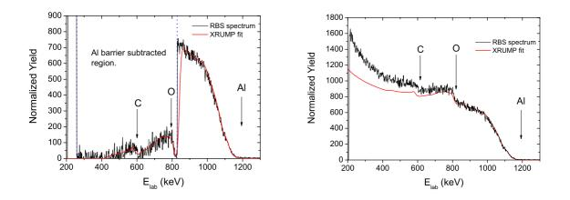
Figure 4.22: Left panel: The 2.0 MeV  ${}^{4}\text{He}^{+}$  backscattering spectrum of the  ${}^{7}\text{Li}$  implanted in Al target measured at  $\theta_{lab}$ =140° (with the Al barrier partially subtracted), and the XRUMP simulated spectrum (red curve). Right panel: Original RBS spectrum, superimposed on the XRUMP fit (red curve).
