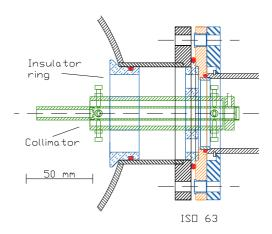
Figure 4.4: Left panel: Photo of collimating system - view from inside the target chamber. Right panel: drawing of the collimating system and insulating supports.
