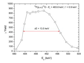
Figure 4.17: The excitation function of the  $^{19}$ F(p, $\alpha\gamma$ ) $^{16}$ O reaction at  $E_{r,lab}$  = 483.6 keV using the LiF-Cu target. The curve through the data points is to guide the eye only.
