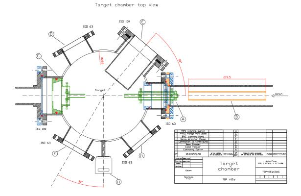
Figure 4.3: Top view drawing of target chamber used at ITN. Colour legend: green – steel AISI 304; orange – other metals; blue – insulator; red – o'rings.
