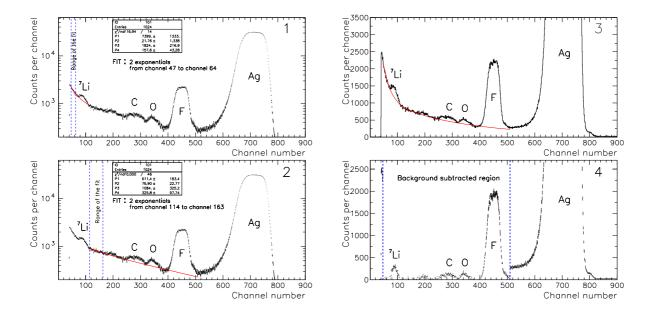
Figure 4.13: The 1.574 MeV  ${}^{4}\text{He}^{+}$  backscattering spectra of the LiF-Ag target, measured at  $\theta_{lab}$ = 115°. Ag plural scattering events (background) subtraction under the  ${}^{7}\text{Li}$ , C, O and F peaks. The background events are fitted with exponentials and then subtracted from the spectrum.
