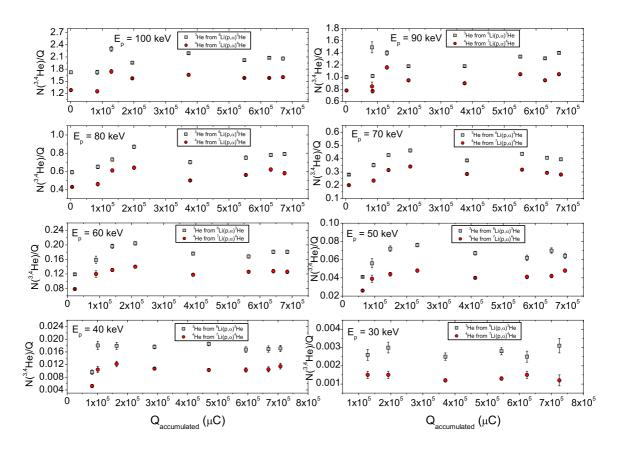
Figure 4.31:  $^7\text{Li}(p,\alpha)^4\text{He}$  yield  $[N(^4\text{He})/Q]$  (red circles) and  $^6\text{Li}(p,\alpha)^3\text{He}$  yield  $[N(^3\text{He})/Q]$  (gray squares) evolution with accumulated charge for the  $Pd_{94.1\%}Li_{5.9\%}$  target. The error bars come from the statistical error on  $N(^{3,4}\text{He})$  counts.
