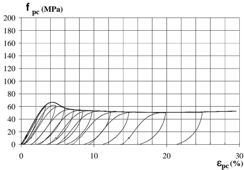
**Fig. 13:** Compression diagram stress – strain of sample e1
