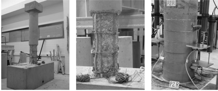
**Fig. 1:** Details of the intervention area on the P2R column, before, during and after the retrofitting with polymer concrete.
