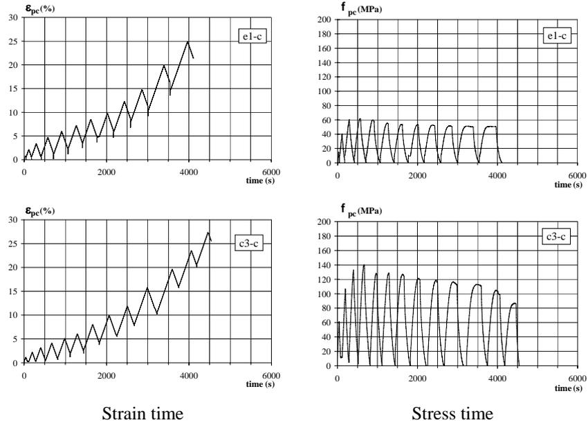
**Fig. 6:** Strains and stress time history (resin samples e1 and c3)
