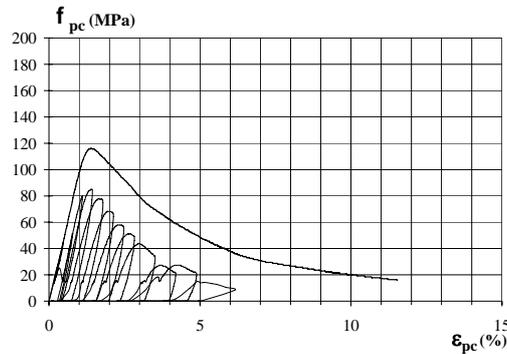
**Fig. 9:** Compression diagram stress – strain of sample a2
