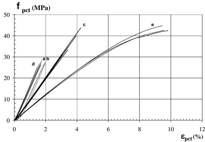
**Fig. 3: Resin and polymer concrete diagrams tension stress – strain in bending**
