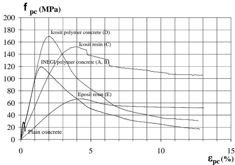
Fig. 14: Compression tests of polymer concrete and their comparison with correspondent curves of plain concrete
