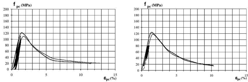
**Fig. 10:** Compression diagrams stress – strain of samples b1 and b2
