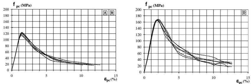
**Fig. 5:** Monotonic compression diagrams of stress–strain of polymer concrete (A, B and D series)
