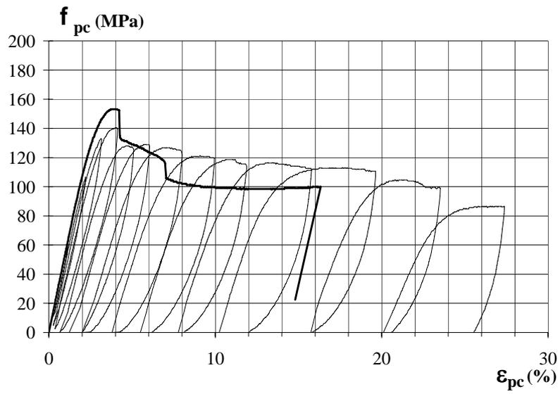
Fig. 11: Compression diagram stress – strain of sample c3
