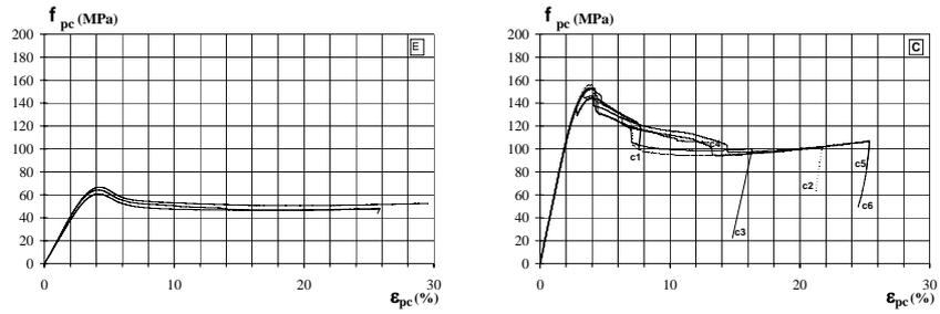
**Fig. 4:** Monotonic compression stress – strain of resin (E and C series)
