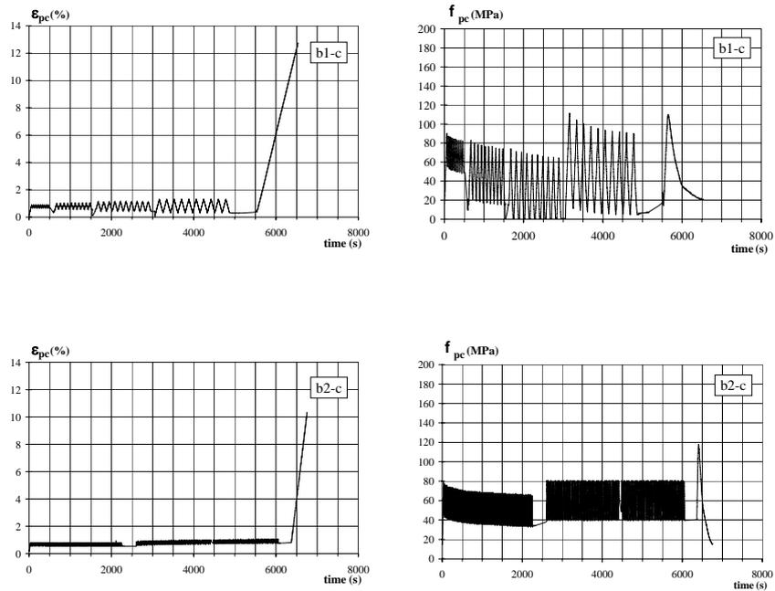
**Fig. 8:** Strains and stress time history (resin samples b1 and b2)
