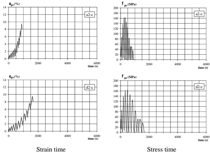
**Fig. 7:** Strains and stress time history (polymer concrete samples a2 and d2)
