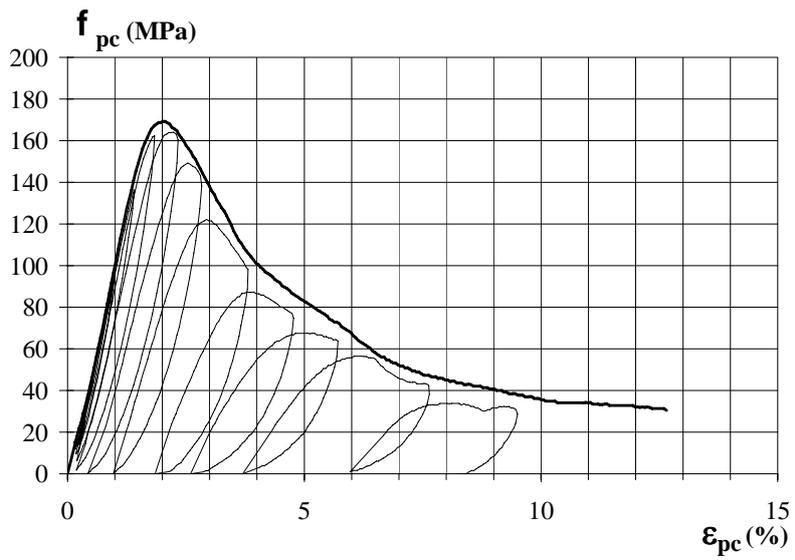
Fig. 12: Compression diagram stress – strain of sample d1
