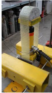
Figure 8: Shear test apparatus.
