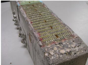
Figure 2: Bottom view of location of strain gauges in bending tests.
