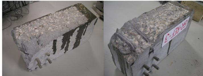
Figure 5: Post-failure surface of the reference specimens.
