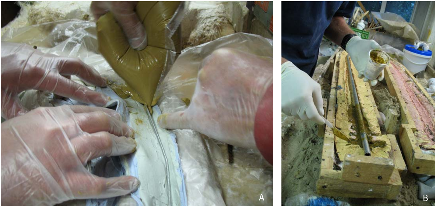
Fig. 13 – Casting: A – using a pouch as a pastry bag containing polyester resin; notice the piece of steel wire inside the mould, providing a rigid structure to the cast. B – applying polyester resin; this layer serves as the base colour for the subsequent painting (photos by Pedro Viegas).
