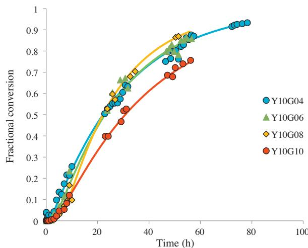
**Fig. 5.** Acetalization of phenylacetaldehyde and glycerol catalyzed by PVA/H-USY composite membranes. Conversion profiles obtained for membranes with increasing cross-linking degrees.
