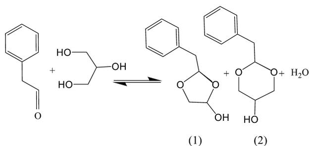
**Scheme 1.** Acetalization of phenylacetaldehyde with glycerol. (1) 2-Benzyl-4-hydroxy methyl-1,3-dioxane. (2) 2-Benzyl-5-hydroxy-1,3-dioxane.
