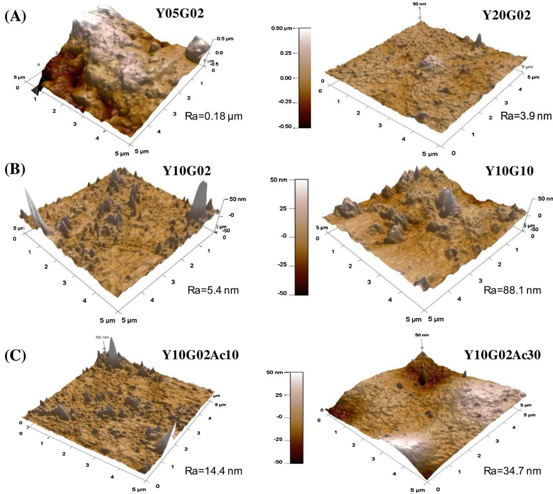
**Fig. 4.** 3D AFM images of PVA membranes with different: (A) catalyst loading (H-USY zeolite); (B) crosslinking degree; (C) acetylation degree.
