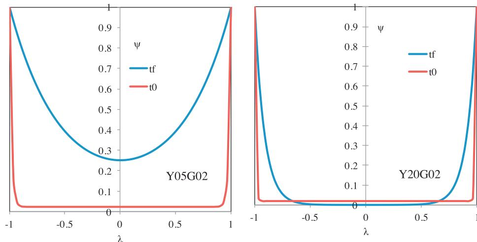
**Fig. 8.** Membrane phenylacetaldehyde concentration profiles calculated assuming symmetrical homogeneous membranes, for the membranes with the lowest (Y05G02) and the highest (Y20G02) zeolite loading, at the initial reaction time ( $t_0$ ) and the final reaction time ( $t_f$ ).
