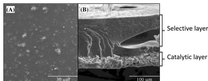
**Fig. 3.** SEM micrographs of Y10G02: (A) surface of the selective layer side; (B) cross section.
