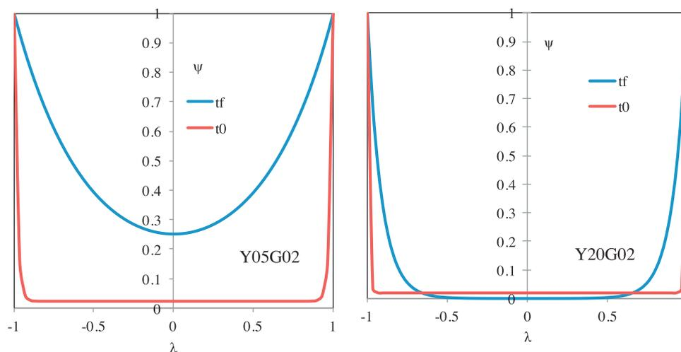
Fig. 8. Membrane phenylacetaldehyde concentration profiles calculated assuming symmetrical homogeneous membranes, for the membranes with the lowest (Y05G02) and the highest (Y20G02) zeolite loading, at the initial reaction time ( $t_0$ ) and the final reaction time ( $t_f$ ).
