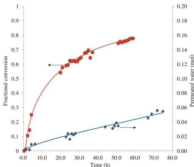
**Fig. 11.** Conversion and permeated water profiles obtained in the pervaporation assisted membrane reactor equipped with membrane Y20G02.
