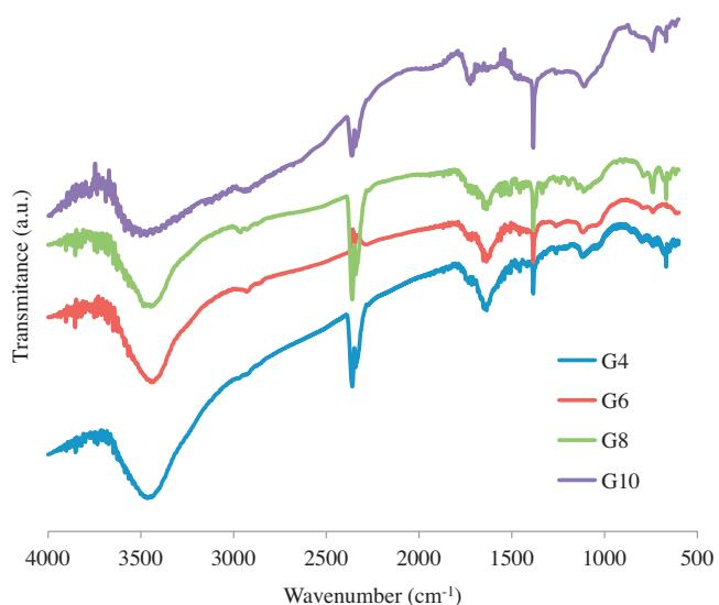
**Fig. 1.** FTIR spectra of membranes Y10G04, Y10G06, Y10G08 and Y10G10. Effect of glutaraldehyde addition.
