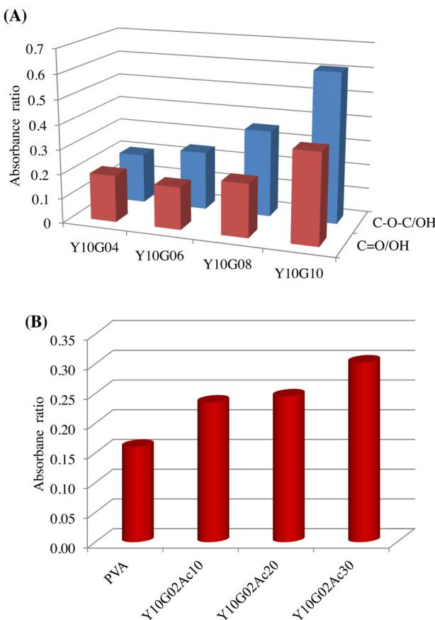
**Fig. 2.** Absorbance ratio between the bands assigned to acetal (C-O-C) or carbonyl groups (C=O) and OH groups: (A) PVA membranes with different polymer cross-linkings (C-O-C/OH); (B) PVA membranes with different acetylation degrees (C=O/OH).
