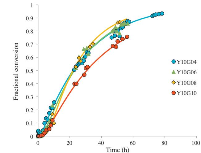
Fig. 5. Acetalization of phenylacetaldehyde and glycerol catalyzed by PVA/H-USY composite membranes. Conversion profiles obtained for membranes with increasing cross-linking degrees.
