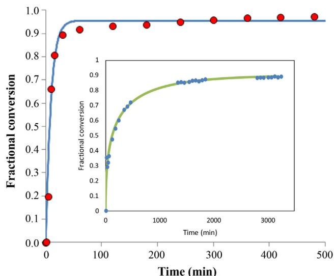
**Fig. 6.** Acetalization of phenylacetaldehyde and glycerol catalyzed by free H-USY at 100 °C and using 99% pure glycerol. Fitting of the LH-SR kinetic model to experimental data. The insertion corresponds to the same reaction carried out at 70 °C and using 87% pure glycerol.
