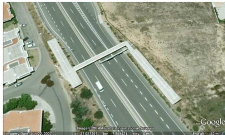
The structure is a simply supported reinforced concrete footbridge, having a span of 29m and a vertical clearance of 5.4m.
