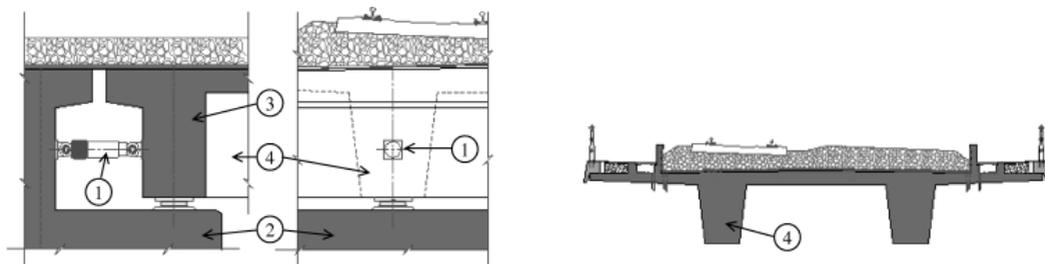
Legend: 1. SMA device, 2. Abutment, 3. Transverse girder, 4. Main girder
