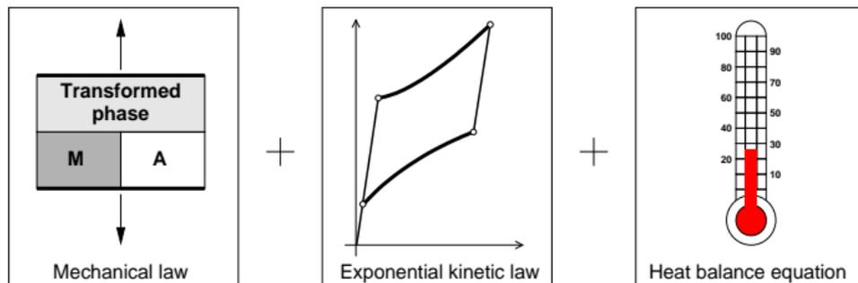
The model couples the constitutive relations, a kinetic law that describes the volume fraction of austenite and a balance equation that considers the thermal effects on the material  $\Rightarrow$  **reliable constitutive model even for high strain rates.**
