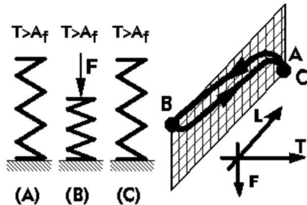
The sample is strongly deformed at relatively low stresses (A to B) at a temperature above  $A_f$ . During subsequent unloading a complete shape recovery occurs (B to C).
