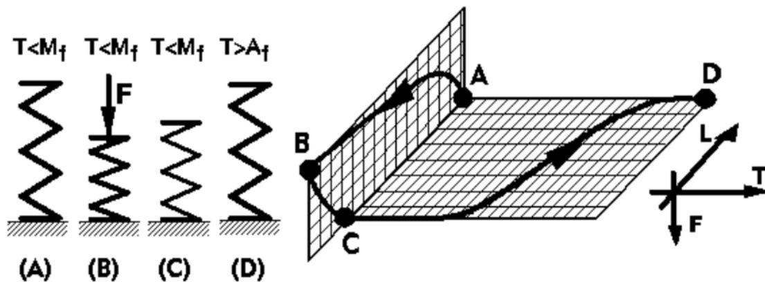
The sample is deformed (A to B) and unloaded (B to C) at a temperature below  $M_f$ . The residual deformation is restored during heating to a temperature above  $A_f$ .
