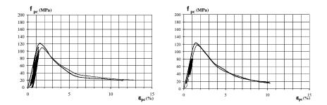
Fig. 10: Compression diagrams stress – strain of samples b1 and b2
