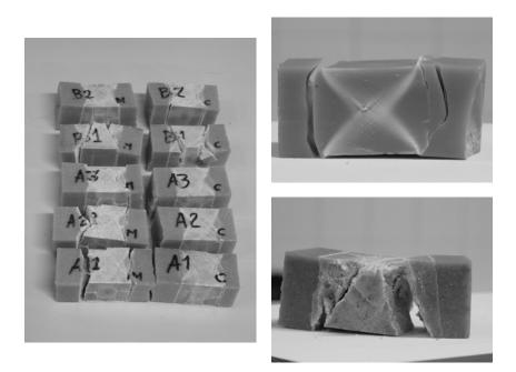
Fig. 2: Details of the samples' rupture after the tests
