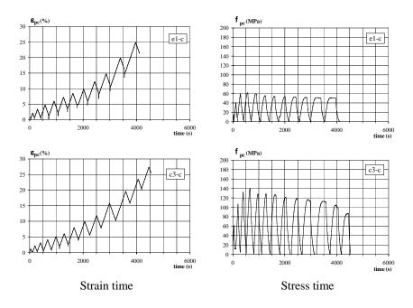
Fig. 6: Strains and stress time history (resin samples e1 and c3)
