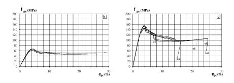
Fig. 4: Monotonic compression stress – strain of resin (E and C series)
