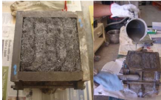
Figure 9: Execution of fibre reinforced grout cubic specimens
