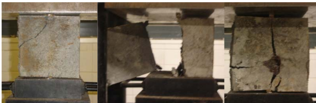
Figure 10: Splitting Test - Failure mode of fibre reinforced grout cubic specimens
