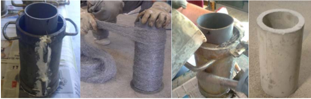
Figure 6: Execution of fibre reinforced grout tubular specimens of circular cross-section
