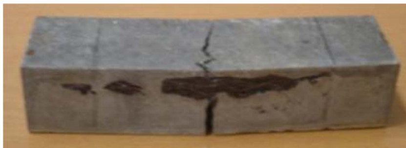
Figure 2: Deficiencies in a specimen (4% fibre vol.; w/c = 0.28)
