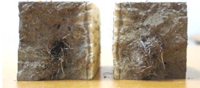
Figure 1: Deficiencies in a specimen (5% fibre vol.; w/c = 0.40)
