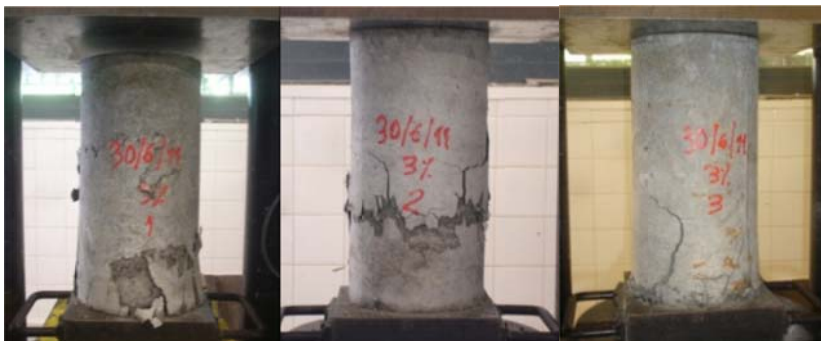
Figure 8: Compressive failure mode of fibre reinforced grout tubular specimens
