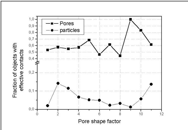
Figure 5 – Fractions of pores (reported to the number of pores of the same pore shape factor class) and of particles (reported to the overall particle population) effectively participating in pore/shape contacts, as a function of pore shape factor.
