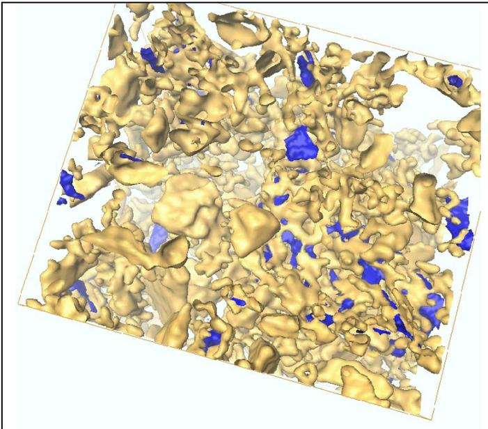
Figure 1 – Reconstructed tomographic image of a 200 x 200 x 200 voxels ( $0.19^3 \mu\text{m}^3$ ) VOI, showing the reinforcing SiC particles, in yellow, and revealing the presence of porosity, in blue.
