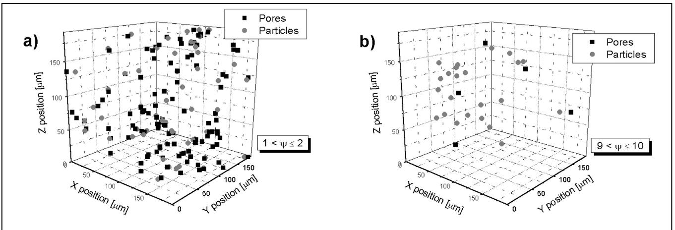
Figure 6 – Three-dimensional plots representing the populations of pores and particles in contact with each other for a given interval of  $\psi$  values. Each object is represented through the position of its centroid, contour representation being omitted. a)  $1 < \psi \leq 2$ ; b)  $9 < \psi \leq 10$ .
