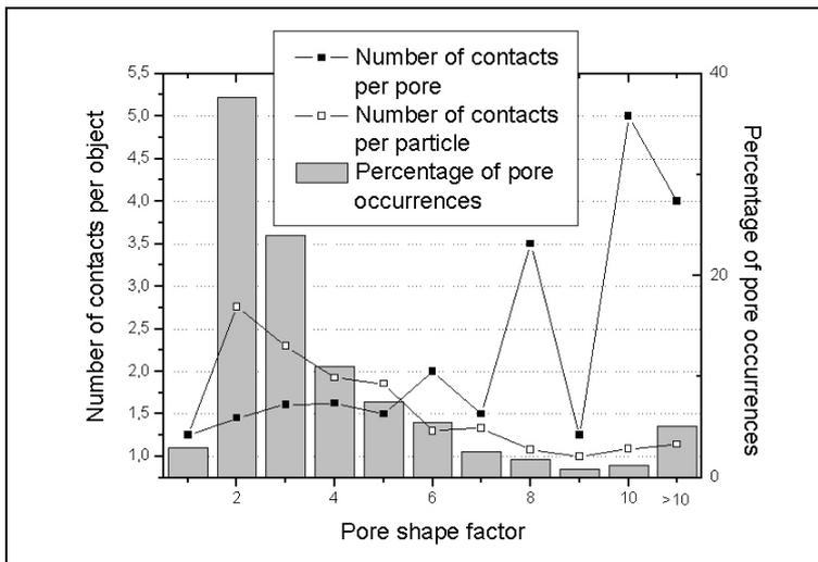
Figure 4 – The figure correlates the pore shape distribution, as the number of pore occurrences for each pore shape factor class, with the number of contacts per pore effectively touching one or more particles, and with the number of contacts per particle effectively touched by pores of that class.
