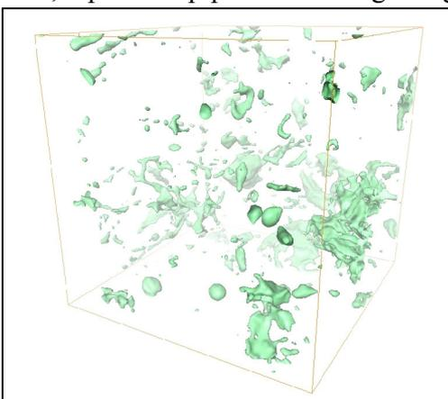
Figure 2 – Another reconstructed tomographic image of a 200 x 200 x 200 voxels ( $0.19^3 \mu\text{m}^3$ ) VOI, this time showing some of the pores occurring in the material, but omitting visualisation of the SiC particles.
