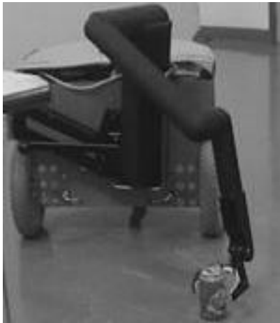
Figure 1: ARPH - Assistant Robot for Handicapped People
