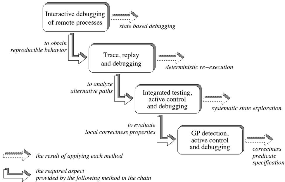
Figure 5.7: Distributed debugging methodologies
