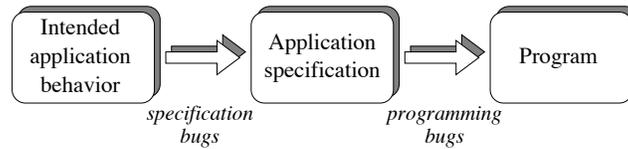
Figure 5.1: Specification and programming bugs
