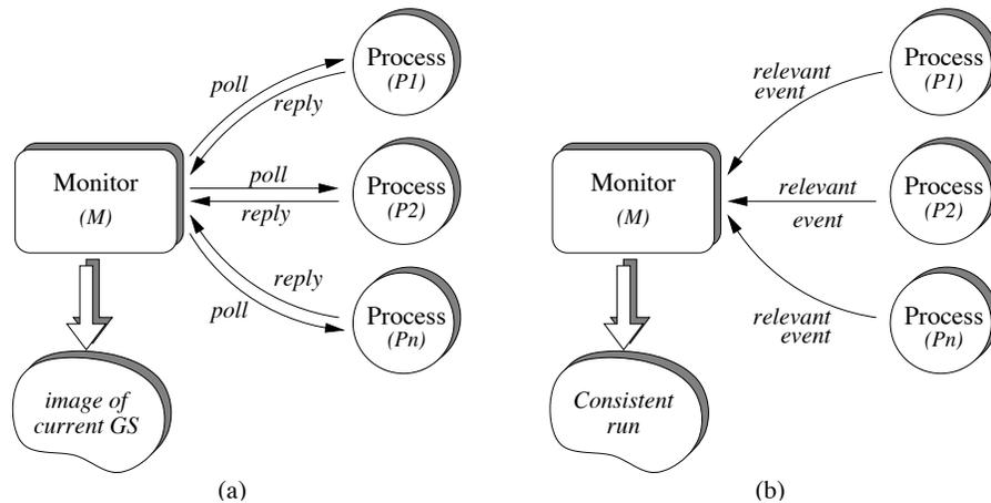
Figure 5.6: Two observation approaches: (a) Global snapshot (b) Active notification
