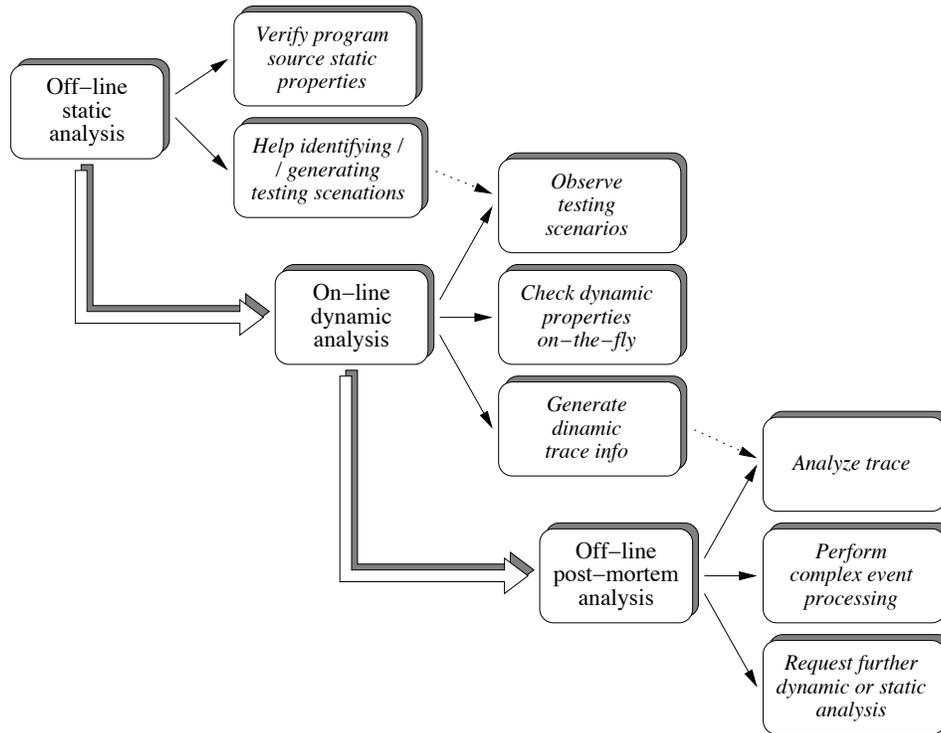
Figure 5.8: Program analysis and debugging at distinct phases of development
